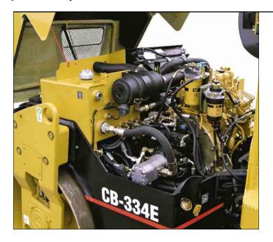
**Engine Enclosure.** Fiberglass engine enclosure pivots upward and locks open with a prop rod.
