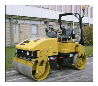
**Increased Production.** The CB-334E XW is equipped with 1400 mm wide drums and can cover greater mat widths in fewer overlapping passes. The rolling pattern changes with an increased production.
