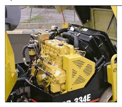
**Power.** The liquid cooled Caterpillar 3024 engine provides a gross power of 34.1 kW (46 hp) and a torque of 143 Nm for excellent performance and reliability on grades and in tough conditions.
