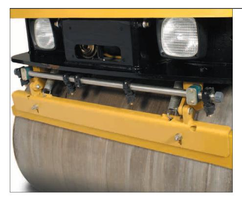
**Spray capabilities.** Constant or intermittent spray capabilities provide extended operation between refills.
