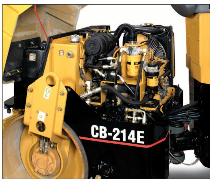
**Engine enclosure.** Fiberglass engine enclosure pivots upward and locks open with a prop rod.
