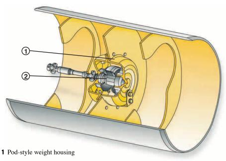
**Pod-style weight housings.** They are assembled and sealed at the factory to ensure cleanliness, extended bearing life and easy field exchange/service.
